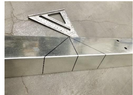
Figure 4: Marking the cut lines for making a corner
